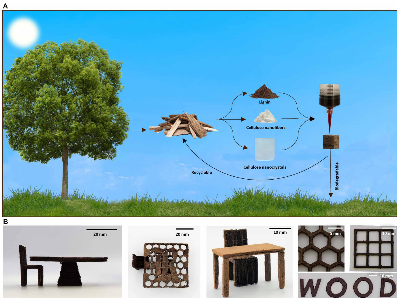
Fig. 1. Process schematic showing 3D printing of wood architectures. (A) Schematic of the wood printing process. (B) Printed samples of various architectures. From the left: A one-legged table with a chair, top view of the table showing a honeycomb architecture with the Rice University R logo in the middle, the chair behind a four-legged table (legs printed and assembled separately), top views of a honeycomb, a rectilinear structure, and the letters WOOD.
