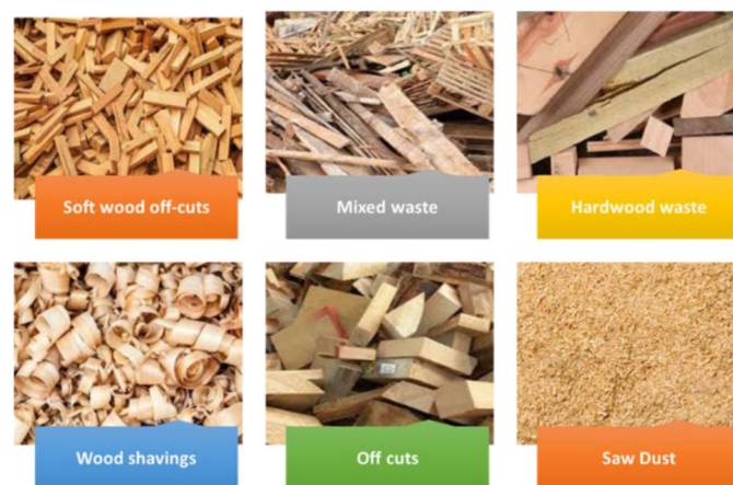
Figure 5. Various forms of wood waste. Adapted from Jahan et al. [5] (open access).
