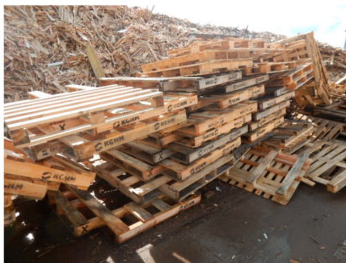
Figure 21. Waste pallets used for PB production. Adapted from Iždinský et al. [162] (open access).
